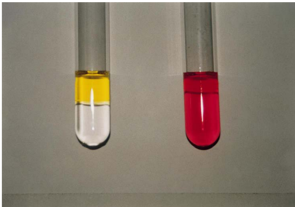
Fig. 2. Partitioning behavior of methyl orange in aqueous two-phase systems. Methyl orange is yellow in the anionic form and is red in amphoteric form.
